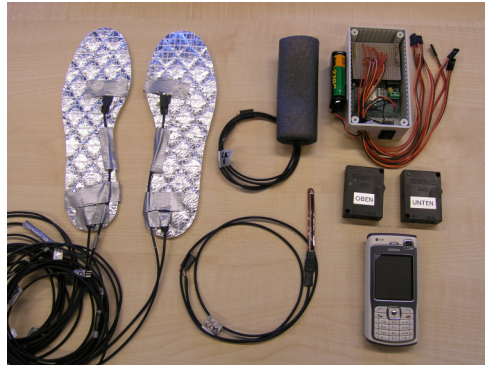
Figure 2: The wireless prototype to sense the rider's motions on the snowboard.
